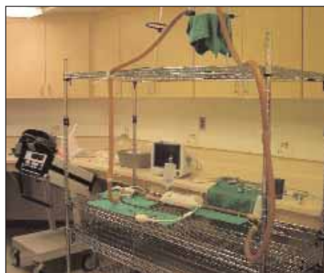
Figure 3. Experimental model of a mock circulatory flow loop assembled to measure vessel wall and vascular prosthesis properties and behavior in different hemodynamic circumstances.
