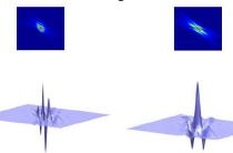
Figure 1. Directional filters of shearlet.
