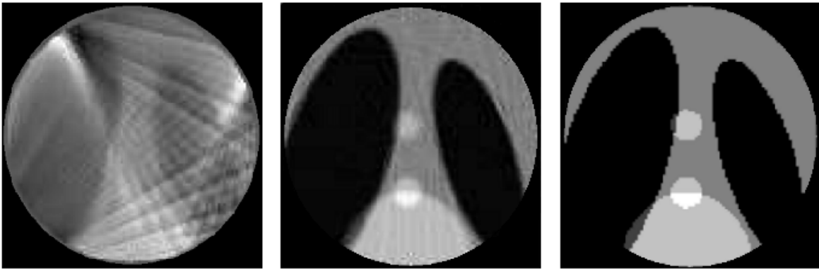
Fig. 7. Visual comparison of ROI reconstruction for the Shepp-Logan phantom using simulated spiral acquisition. A representative 2D slice is shown. From left to right: unregularized reconstruction; regularized ROI CT reconstruction; ground truth
