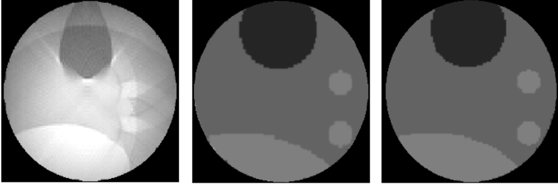
Fig. 6. Visual comparison of ROI reconstruction for the Shepp-Logan phantom using simulated spherical acquisition. A representative 2D slice is shown. From left to right: unregularized reconstruction; regularized ROI CT reconstruction; ground truth
