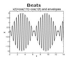
In acoustics, a beat is an interference between two sounds of slightly different frequencies, perceived as periodic variations in volume whose rate is the difference between the two frequencies.
