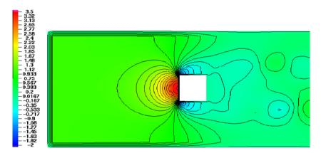
Fig. 13. Problem Q2 (Re = 100): The midplane pressure contours around a square cylinder. The solution shown was computed with  $h_{\text{max}} = 1/256$  and  $h_{\text{min}} = 1/1024$  at t = 16.
