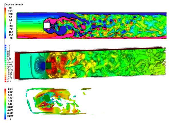
**Fig. 16.** Channel flow around a square cylinder at Re = 1000: Spanwise vorticity for the midplane y = 0.205. Pressure isosurfaces and vorticity isosurface  $|\mathbf{w}| = 100$  colored by the absolute velocity. The plots illustrate solution computed with  $h_{\text{max}} = 1/256$  and  $h_{\text{min}} = 1/1024$  at t = 8. (For interpretation of the references to color in this figure legend, the reader is referred to the web version of this article.)
