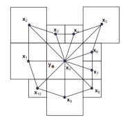
**Fig. 5.** Left: Reference points for the diffusion flux approximation; Right:  $u_h(\mathbf{y})$  is defined by a linear interpolation based on the fan triangulation with the center in  $\mathbf{x}_V$ , i.e. interpolation of  $u_h(\mathbf{x}_V)$ ,  $u_h(\mathbf{x}_1)$ ,  $u_h(\mathbf{x}_1)$ ,  $u_h(\mathbf{x}_1)$ , in this example.
