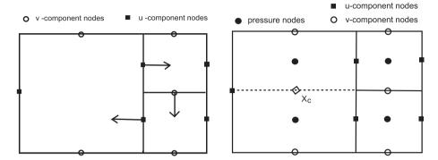
Fig. 3. Left: A single local div-free mode, which is subgrid for the coarse grid cell. Right: Introducing additional pressure d.o.f. for the coarse cell next to fine cells. This yields a stronger discrete div-free condition and precludes the occurrence of subgrid div-free modes such as shown in the left figure.
