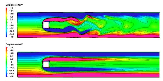
**Fig. 12.** Problem Q2 (Re = 100): Spanwise vorticity at time t = 16 for the midplane y = 0.205. The top plot shows the development of vortex street for solution by BDF2 with FD advective terms; the bottom plot shows an over-diffusive solution computed by BDF2 with semi-Lagrangian method (linear interpolation). Both solutions were computed with  $h_{\text{max}} = 1/256$  and  $h_{\text{min}} = 1/1024$  at t = 16.
