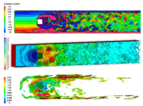
**Fig. 17.** Channel flow around a square cylinder at Re = 10000: Spanwise vorticity for the midplane y = 0.205. Pressure isosurfaces and vorticity isosurface  $|\mathbf{w}| = 100$  colored by the absolute velocity. The plots illustrate solution computed with  $h_{\text{max}} = 1/256$  and  $h_{\text{min}} = 1/1024$  at t = 8. (For interpretation of the references to color in this figure legend, the reader is referred to the web version of this article.)
