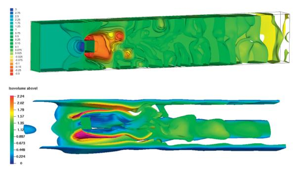
**Fig. 15.** Problem Q2 (Re = 100): Pressure isosurfaces and vorticity isosurface |**w**| = 20 colored by the absolute velocity. The plots illustrate solution computed with  $h_{\text{max}} = 1/256$  and  $h_{\text{min}} = 1/1024$  at t = 16. (For interpretation of the references to color in this figure legend, the reader is referred to the web version of this article.)
