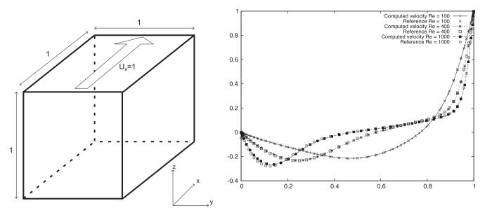
**Fig. 6.** Left: The 3D driven cavity problem setup; Right: The centerline  $((0.5, 0.5, z), 0 \le z \le 1)$  *u*-velocities compared to reference data from [33].
