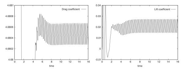
**Fig. 11.** The evolution of drag (left) and lift (right) coefficients for the flow around a square cylinder with Re = 100 (problem Q2) computed with  $h_{max} = 1/32$ ,  $h_{min} = 1/1024$ .
