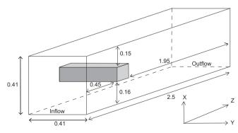
Fig. 9. Computational domain for flow around a cylinder with square cross-section.
