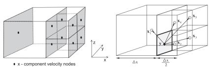
Fig. 1. Left: Each shared face holds a node for velocity x-component. The nodes are located at faces barycenters. Right: Discretization stencil for  $\partial p/\partial x$ .
