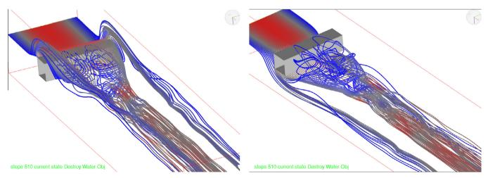
**Fig. 14.** Problem Q2: Streamlines of the developed flow around a square cylinder for Re = 100. The streamlines are selected for two fluid layers entering the domain slightly above and below x = 0.21.
