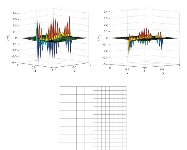
**Fig. 2.** The velocity error is dominated by the div-free modes occurring on the coarse-to-fine grids interface. The left figure shows the u-component of the error, the right figure shows the v-component, and the bottom figure shows the grid for h = 1/8.
