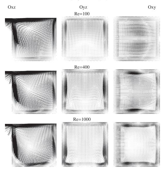
Fig. 8. The 2D planar projections of steady state velocity fields at the midplanes for the 3D driven cavity problem with Re = 100, 400, 1000.
