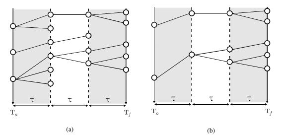
**Figure 2:** (a) Illustration of the GKLT algorithm and (b) assembly of *N* backward trajectories. Although shifts in the distribution of the integral are defined by the resampling time  $\tau$ , reconstruction of backward trajectories allows for estimates on *T*-time averaged trajectories after implementation of GKLT.
