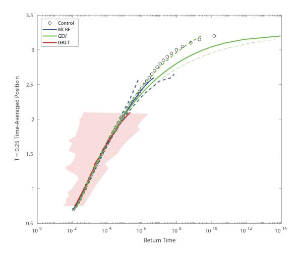
**Figure 5:** Return time estimates for the Ornstein Uhlenbeck process time average observable using GKLT for 4 different *C* values and 100 experiments, GEV, and Monte Carlo brute forces methods with numerical cost  $4 \cdot 10^4$ . Relative error curves for MC brute force and GEV estimates are represented by dashed lines. Relative error estimated by 100 experiments of the GKLT process is represented by the shaded red region.
