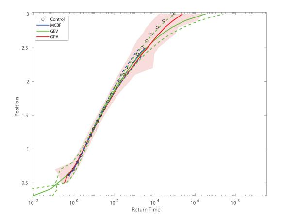
**Figure 9:** Return time estimates for the Ornstein Uhlenbeck process using GPA for 3 different *C* values estimated over 10 experiments, GEV, and Monte Carlo brute forces methods with numerical cost  $3 \cdot 10^3$ . Relative error estimates for GEV amd MC methods (dashed lines) and GPA (red region) are estimated from 10 experiments.
