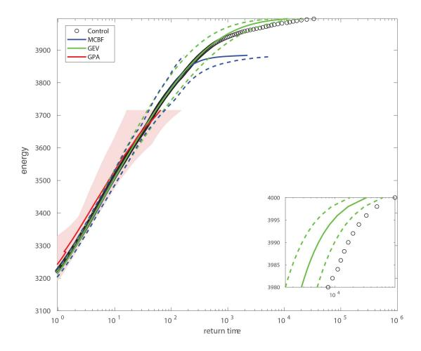
**Figure 14:** Return time estimates for the Lorenz '96 process using GPA for  $C = [3.1 \cdot 10^{-3}, 6.4 \cdot 10^{-3}]$  estimated over 10 experiments for N = 2000 starting particles, GEV, and Monte Carlo brute forces methods with numerical cost  $4 \cdot 10^4$ . Relative error estimates for GEV and MC methods (dashed lines) and GPA (red region) are estimated from 10 experiments.
