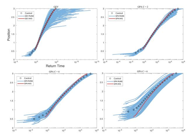
**Figure 13:** Illustration of the deviation of the return time curves from the control for GEV and 3 different tilting *C* values of GPA. Notice that the average return time curve (red) for the GEV fits the control (black  $\circ$ ) for all long return times while accurate estimates for GPA only occur near the optimal threshold value.
