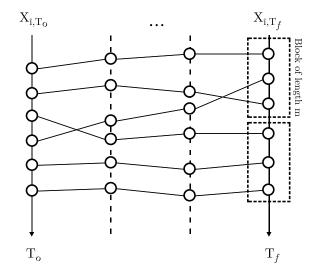
Figure 3: Illustration of the block maxima for GEV to GPA comparison. Many trajectories are run under the dynamics up to the sampling time  $T_f$  and the final values are used to form the block maxima (indicated by dashed boxes).
