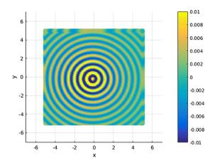
**Fig. 7.** Cross-section z = 0 plot of the generated field, showing outgoing character.
