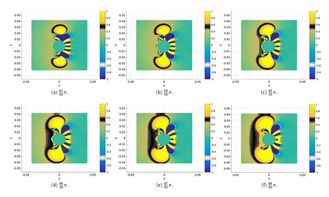
**Fig. 9.** Cross-sectional (z = 0) time snapshots of the propagating generated acoustic field for different values of *kct*. Control region  $D_1$  to the left of the source, with the null region  $D_2$  to the right. (For interpretation of the references to colour in this figure legend, the reader is referred to the web version of this article.)
