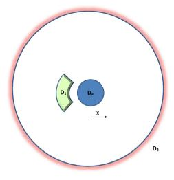
**Fig. 11.** Planar sketch of the geometry showing the source  $D_a$ , the control region  $D_1$  and the far field region  $D_2$ .
