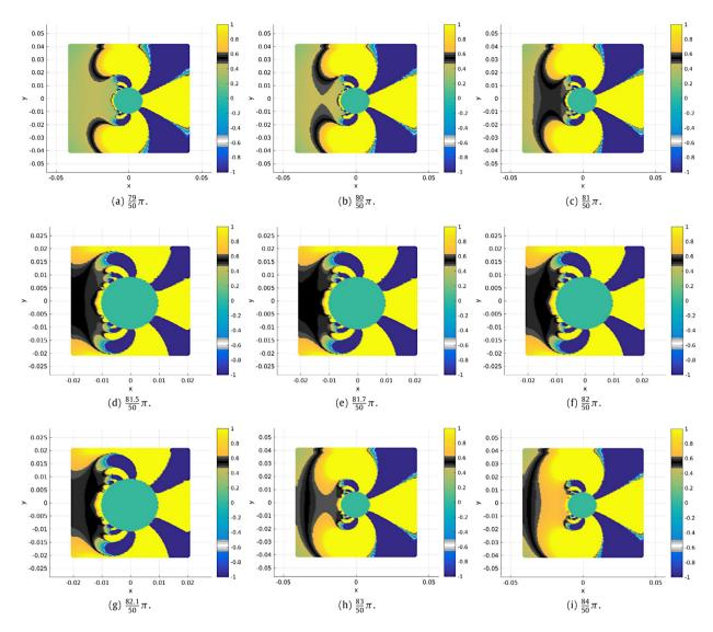
**Fig. 15.** Cross-sectional (z = 0) time snapshots of the propagating generated field for different values of *kct*. Control region  $D_1$  to the left of the source, where an incoming wave is approximated. (For interpretation of the references to colour in this figure legend, the reader is referred to the web version of this article.)
