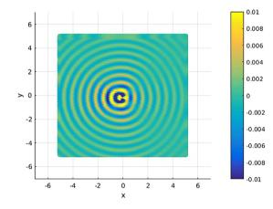
**Fig. 12.** Cross-section z = 0 plot of the generated field, showing outgoing character, with fast radiation decay.
