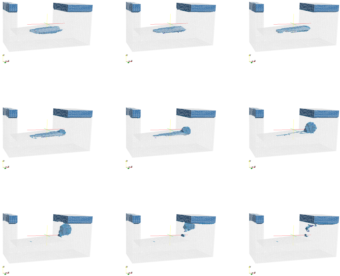
Fig. 16. Numerical simulation of a bubble rising under an inclined plane under gravity forces ( H = 0.0333 ). The angle is equal to 5^\circ degrees. Snapshots of the solution at times t = 0.05, 0.5, 1.0, 1.5, 2.0, 2.25, 2.5, 2.75 and 3.0 s. (top to bottom, left to right).
