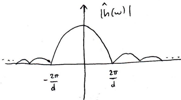
First zero at  $\frac{\omega d}{2} = \pi \Rightarrow \omega = \frac{2\pi}{d}$
