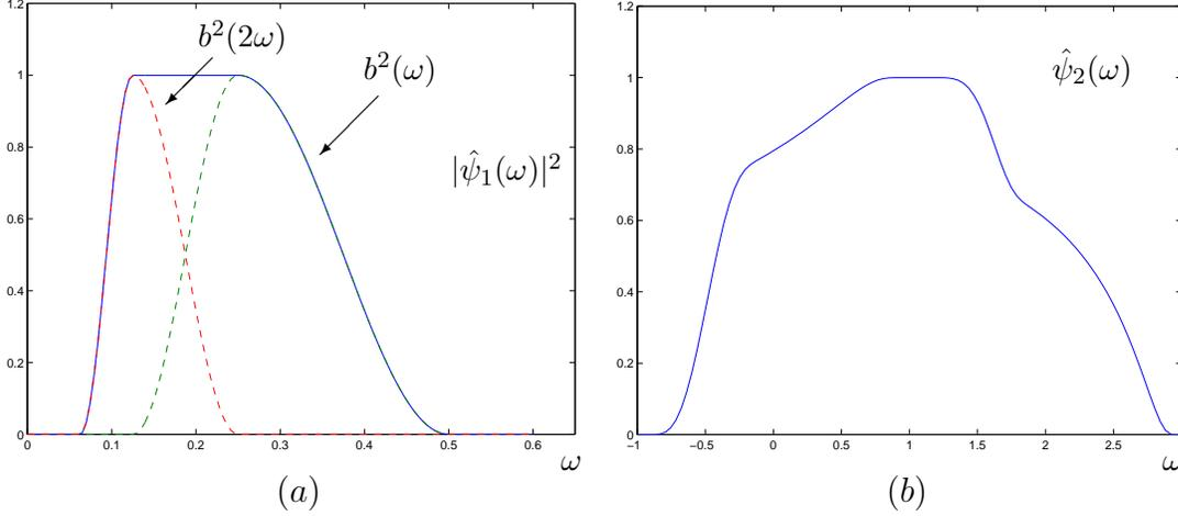
Fig. A.1. (a) The function  $|\hat{\psi}_1(\omega)|^2$  (solid line), for  $\omega > 0$ ; the negative side is symmetrical. This function is obtained, after rescaling, from the sum of the window functions  $b^2(\omega) + b^2(2\omega)$  (dashed lines). (b) The function  $\hat{\psi}_2(\omega)$ .
