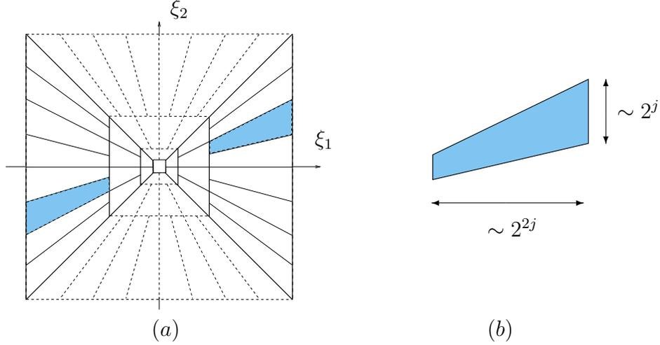
Fig. 1. (a) The tiling of the frequency plane  $\widehat{\mathbb{R}}^2$  induced by the shearlets. The tiling of  $\mathcal{D}_0$  is illustrated in solid line, the tiling of  $\mathcal{D}_1$  is in dashed line. (b) The frequency support of a shearlet  $\psi_{j,\ell,k}$  satisfies parabolic scaling. The figure shows only the support for  $\xi_1 > 0$ ; the other half of the support, for  $\xi_1 < 0$ , is symmetrical.
