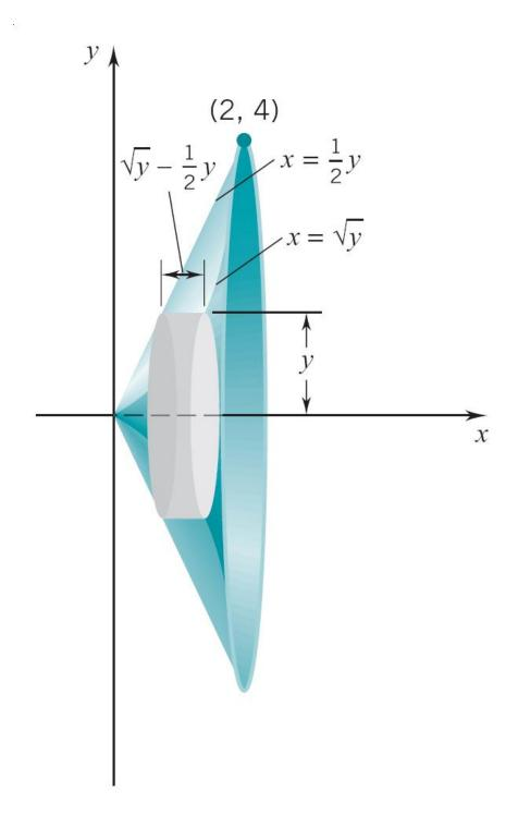
*Example* 8. Find the volume of the solid generated by revolving about the x-axis the region between  $y = x^2$  and y = 2x.
