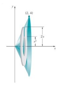
**Example** Example 5. Find the volume of the solid generated by revolving the region between  $y = x^2$  and y = 2x about the y-axis.
