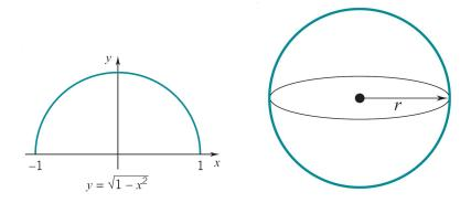
Solid of Revolution About the y-Axis: Disk Cylinder Volume:  $\pi[g(y_i^*)]^2 \Delta y_i$  Riemann Sum:  $\sum \pi[g(y_i^*)]^2 \Delta y_i$
