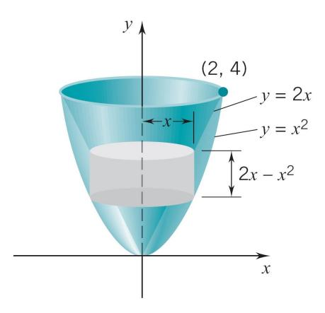
*Example* 7. Find the volume of the solid generated by revolving about the y-axis the region between  $y = x^2$  and y = 2x.
