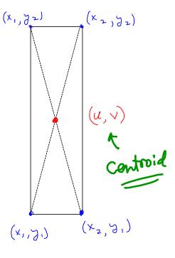
**Question:** Suppose the region on the right is a thin sheet of rigid material. If you were going to place it horizontally flat, and try to balance it on a pin, where should the tip of the pin contact the region?  $(U_{1},V_{1})$
