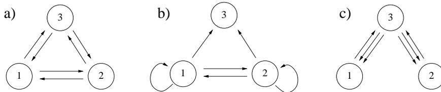
Figure 2. a,b) Examples of three-cell networks in which all cells coevolve: assuming one-dimensional cell dynamics, they cannot support multifrequency oscillations. c) A network in which cell 3 can robustly oscillate at twice the frequency of cells 1 and 2, as only cells 1 and 2 coevolve.
