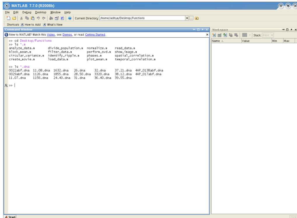
On my computer, all the files (data and MATLAB programs ) are stored in the folder *Functions* on the *Desktop*. Writing *ls* lists all the files in the current directory . Writing *ls \*.dna* lists all the files with an extension *.dna* . MATLAB programs have an extension of *.m*. So typing *ls \*.m* will list all the MATLAB programs in the current directory .
