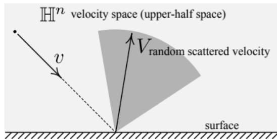
Scattering characteristics of gas-surface interaction encoded in operator  $P$ .
