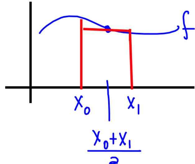
The height of each rectangle is the function value of the  $x$  value at the MIDPOINT of the width of the rectangle.
