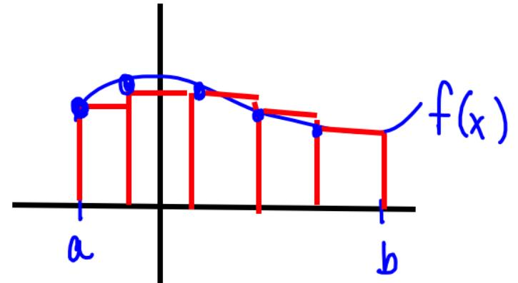
The height of each rectangle is the function value of the x value on the LEFT side of the rectangle.
