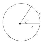
In general, the **radian measure of a central angle**  $\theta$  can be determined by the formula  $\theta = \frac{s}{r}$ , where s is the length of the intercepted arc and r is the radius of the circle and r and s are measured in the same units.
