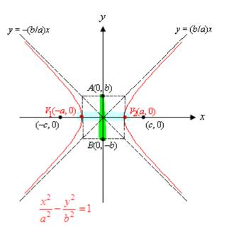
Center: (0,0) Foci: (-c,0) and (c,0), where  $c^2 = a^2 + b^2$ Vertices:  $V_1(-a,0)$  and  $V_2(a,0)$ Transverse Axis:  $\overline{V_1V_2}$  Length of Transverse Axis: 2a Conjugate Axis:  $\overline{AB}$  Length of Conjugate Axis: 2b
