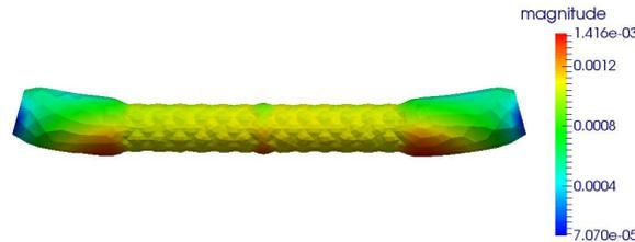
FIG. 10. Deformation of the vessel with two Palmaz-like stents inside.
