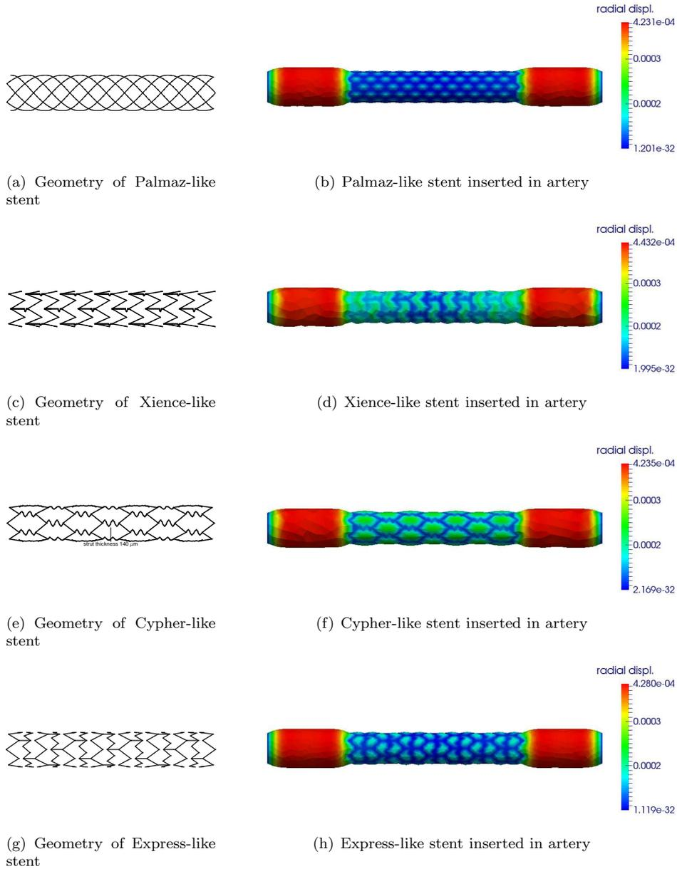
FIG. 6. The figures of the left show the front view of the geometry of middle lines for each of the stents considered. The figures on the right show vessel deformation colored by radial displacement.
