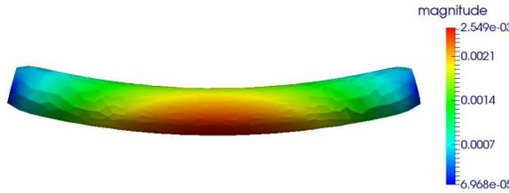
FIG. 8. *Vessel (shell) deformation without a stent, colored by radial displacement. Boundary conditions specified in Data 2 above, causing bending, were used.*
