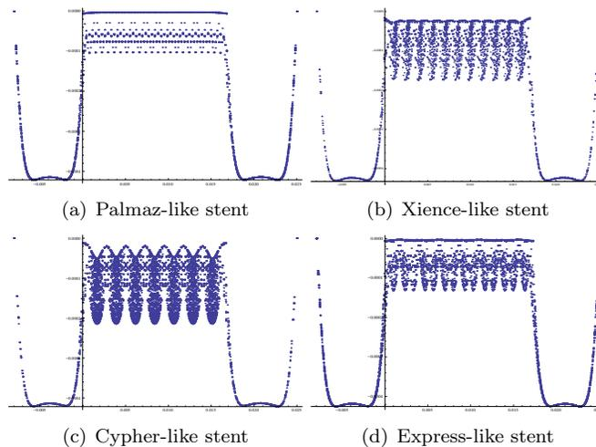
FIG. 7. Radial displacement in terms of mesh points versus horizontal stent axis.
