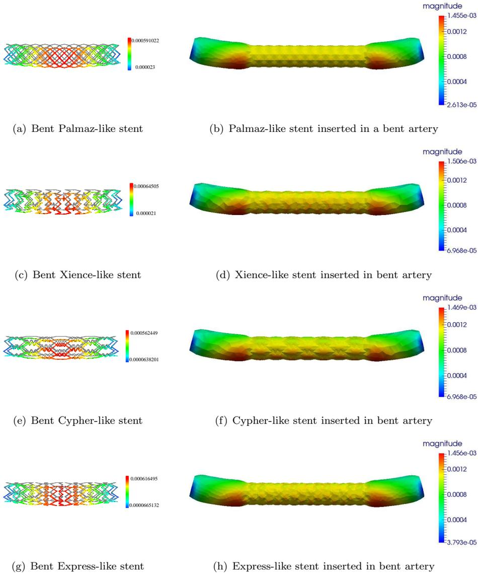
FIG. 9. The figures on the left show the reference (in grey) and bent configuration (colored by radial displacement) for each of the four stents. The figures on the right show deformation of the vessel, colored by radial displacement, with a stent inserted into a bent vessel.
