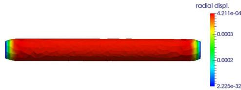
FIG. 5. Vessel (shell) deformation without a stent, colored by radial displacement.
