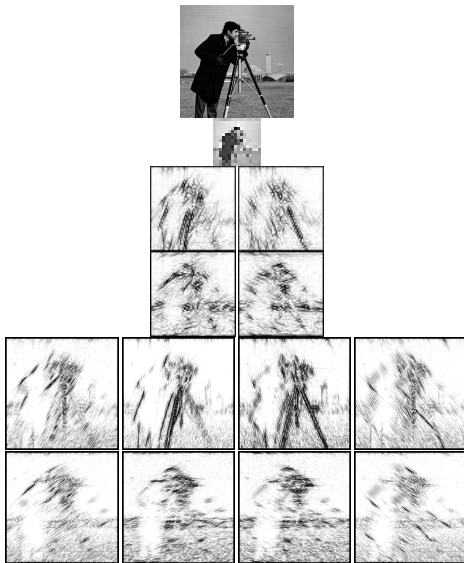
Fig. 3. The top image is the original Cameraman image. The image below the top image contains the approximate shearlet coefficients. Images of the detail shearlet coefficients are shown below this with an inverted grayscale for better presentation.
