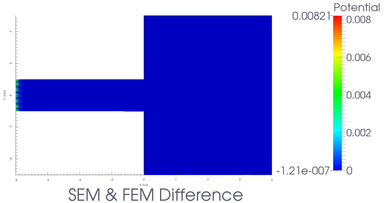
Figure 39: Absolute difference of SEM & FEM solutions. Some difference is revealed on the left boundary.
