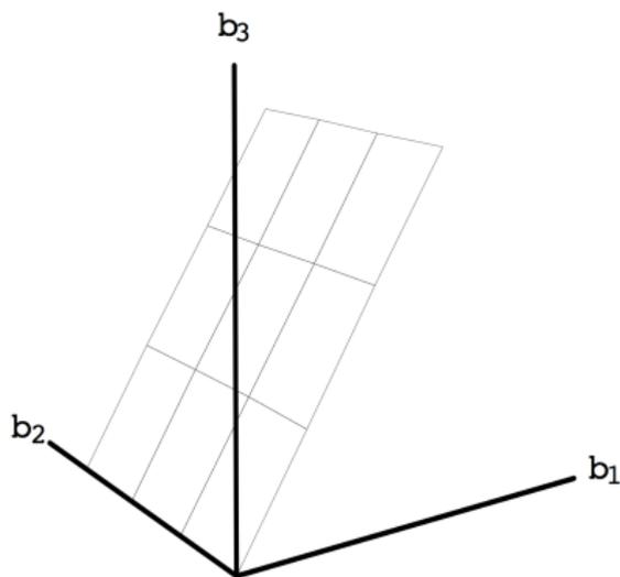
Columns of  $A$  span a plane in  $\mathbb{R}^3$  through  $\mathbf{0}$
