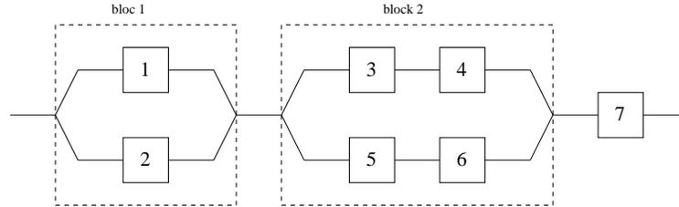
For a subsystem connected in parallel to function, at least one of the components or subsystems in the parallel must work. For a subsystem connected in series to function, all the components or subsystems in the series must work. If the components work independently of one another and  $p_i = P(\text{component } i \text{ works}) = 0.9$  for  $i = 1, \dots, 7$ , calculate  $P(\text{system works})$ .
