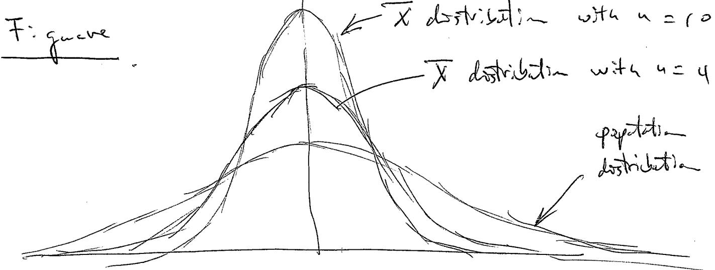
Example: Let  $X_1, X_2, \dots, X_5$  be a random sample from  $N(\mu=1.5, \sigma^2=0.35^2)$ . Then  $\bar{X} \sim N\left(\mu_{\bar{X}}=1.5, \sigma_{\bar{X}}^2=\frac{0.35^2}{5}\right)$
