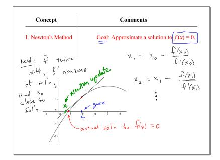
**Example:** Use one iteration of Newton's method from a guess of  $x_0 = 1$  to approximate a solution to  $x^3 - 3x^2 + 2x = 0.1$ . **Popper P20**
