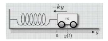
Hooke's law states that for small displacements, the restoring force is proportional to the displacement.
