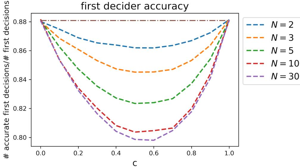
Figure 5.2: Simulation results for first decider accuracy in cliques of size  $N$  with threshold  $\theta = 2$ . The grey dash-dot line gives the expected accuracy for a single decider with threshold  $\theta$ ,  $1/(1 + e^{-\theta})$ . First decider accuracy falls below this benchmark for  $0 < c < 1$ , when deciders may be expected to receive a mix of independent and common observations.
