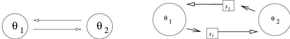
Figure 13: A network consisting of two identical phase oscillators connected directly (left) and through buffer cells (right).
