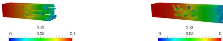
Figure 13—Threshold of the aqueous phase saturation at time  $t = 23$  days (left) and  $t = 37$  days (right). Minimum value is 0.01 and maximum value is 0.1. Case:  $A_{pc} = 10^7$ .
