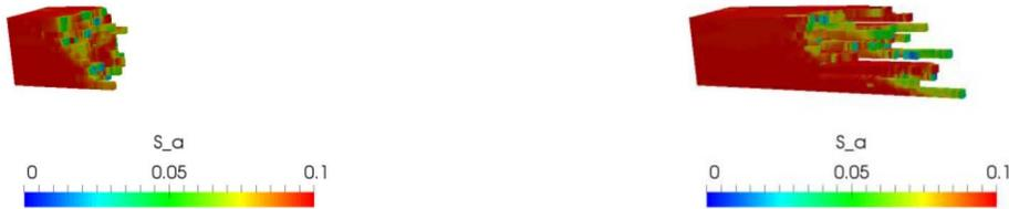
Figure 15—Threshold of the aqueous phase saturation at time  $t = 23$  days (left) and  $t = 37$  days (right). Minimum value is 0.01 and maximum value is 0.1. Case:  $A_{pc} = 10^5$ .
