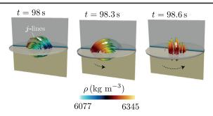
FIG. 5. Emergence of a rotating gravity wave in Ga and GaInSn eutectic (miscible) setup,  $J = 1.5 \times 10^5 \text{ A m}^{-2}$ . We show the isosurface  $\rho = (\rho_1 + \rho_2)/2$ , the density  $\rho$  in color code in the vertical plane x = 0, and lines of excess current j.
