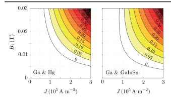
FIG. 2. Growth rate  $\lambda$  in s<sup>-1</sup> of the fundamental wave (m = 1,  $\kappa_{11} = 1.841$ ) in the J- $B_z$  plane in a  $R = H_1 = H_2 = 2$  cm setup with layers of Ga and Hg or Ga and GaInSn eutectic.
