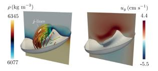
FIG. 6. Simulation with Ga and GaInSn eutectic (miscible setup) using exaggerated diffusion  $D_{\rm fake} = 100D = 1.7 \times 10^{-7} \, {\rm m^2 \, s^{-1}};$   $J = 4 \times 10^5 \, {\rm A \, m^{-2}}; \ t = 31.35 \, {\rm s}.$  The interface shown here is the isosurface  $\rho = (\rho_1 + \rho_2)/2$ .
