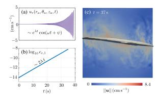
FIG. 4. Simulations in the immiscible Ga and Hg setup. (a) Time series of the velocity at  $r_a = 0$ ,  $\theta_a = 0$ ,  $z_a = -5$  mm gives  $\omega$ . (b) Time series of  $e_{c,1}$  gives  $\lambda$  ( $e_{c,1}$  is the kinetic energy of the azimuthal Fourier mode m = 1). (c) Isosurface  $\rho = (\rho_1 + \rho_2)/2$  and turbulent structures in the vertical plane x = 0 at t = 37 s.
