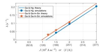
FIG. 3. Growth rate  $\lambda$  in s<sup>-1</sup> of the fundamental wave (m=1,  $\kappa_{11}=1.841$ ) as a function of J or I in a  $R=H_1=H_2=2$  cm setup with magnetic field  $B_z=15$  mT.
