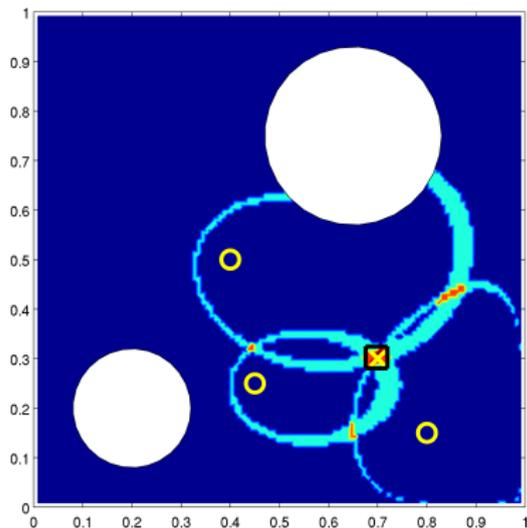
Example: source identification with known intensity  $V(\mathbf{y}) = \mathbf{d}/\mathbf{a}$ . Source position is an intersection of  $(d_i/a)$ -level sets of  $v^{(i)}$ .
