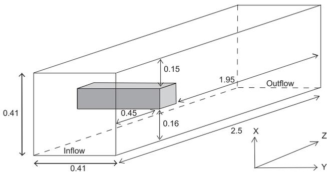
Fig. 9. Computational domain for flow around a cylinder with square cross-section.
