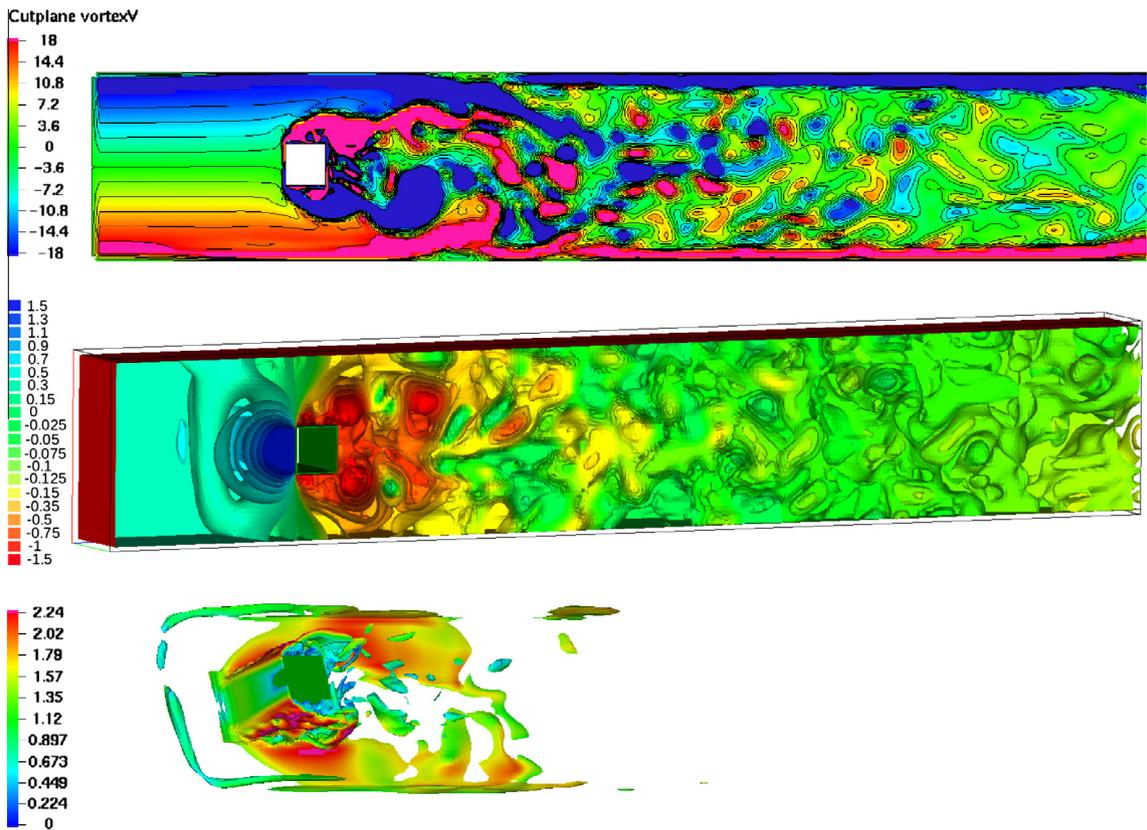
Fig. 16. Channel flow around a square cylinder at  $Re = 1000$ : Spanwise vorticity for the midplane  $y = 0.205$ . Pressure isosurfaces and vorticity isosurface  $|\mathbf{w}| = 100$  colored by the absolute velocity. The plots illustrate solution computed with  $h_{\max} = 1/256$  and  $h_{\min} = 1/1024$  at  $t = 8$ . (For interpretation of the references to color in this figure legend, the reader is referred to the web version of this article.)
