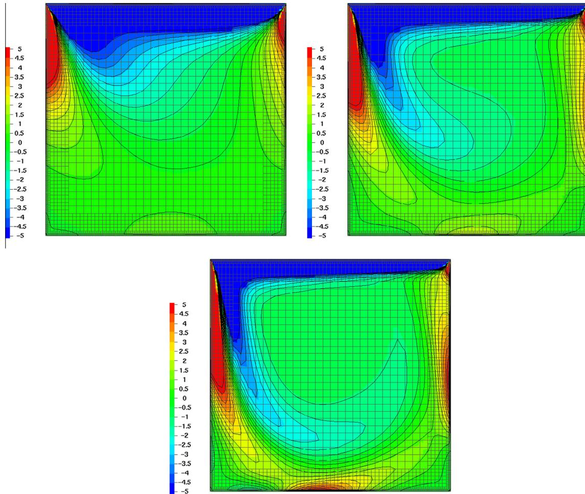
Fig. 7. Spanwise vorticity for the midplane  $y = 0.5$  and  $Re = 100$  (left),  $Re = 400$  (right),  $Re = 1000$  (bottom).
