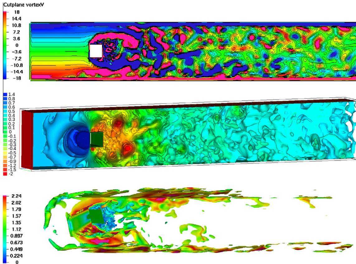
**Fig. 17.** Channel flow around a square cylinder at  $Re = 10000$ : Spanwise vorticity for the midplane  $y = 0.205$ . Pressure isosurfaces and vorticity isosurface  $|w| = 100$  colored by the absolute velocity. The plots illustrate solution computed with  $h_{\max} = 1/256$  and  $h_{\min} = 1/1024$  at  $t = 8$ . (For interpretation of the references to color in this figure legend, the reader is referred to the web version of this article.)
