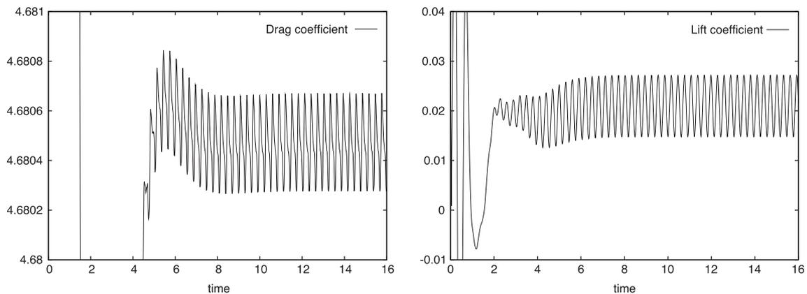
Fig. 11. The evolution of drag (left) and lift (right) coefficients for the flow around a square cylinder with  $Re = 100$  (problem Q2) computed with  $h_{max} = 1/32$ ,  $h_{min} = 1/1024$ .
