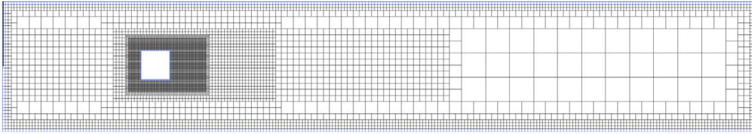
Fig. 10. The cutaway of the grid at  $y = 0.205$  for  $h_{max} = 1/32$  and  $h_{min} = 1/1024$ .
