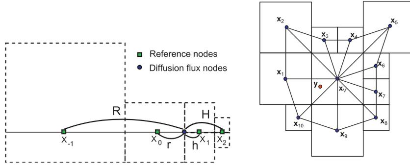
Fig. 5. Left: Reference points for the diffusion flux approximation; Right:  $u_h(\mathbf{y})$  is defined by a linear interpolation based on the fan triangulation with the center in  $\mathbf{x}_V$ , i.e. interpolation of  $u_h(\mathbf{x}_V)$ ,  $u_h(\mathbf{x}_1)$ ,  $u_h(\mathbf{x}_{10})$  in this example.
