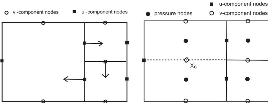
**Fig. 3.** Left: A single local div-free mode, which is subgrid for the coarse grid cell. Right: Introducing additional pressure d.o.f. for the coarse cell next to fine cells. This yields a stronger discrete div-free condition and precludes the occurrence of subgrid div-free modes such as shown in the left figure.
