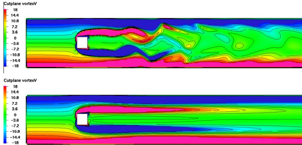
**Fig. 12.** Problem Q2 ( $Re = 100$ ): Spanwise vorticity at time  $t = 16$  for the midplane  $y = 0.205$ . The top plot shows the development of vortex street for solution by BDF2 with FD advective terms; the bottom plot shows an over-diffusive solution computed by BDF2 with semi-Lagrangian method (linear interpolation). Both solutions were computed with  $h_{\max} = 1/256$  and  $h_{\min} = 1/1024$  at  $t = 16$ .
