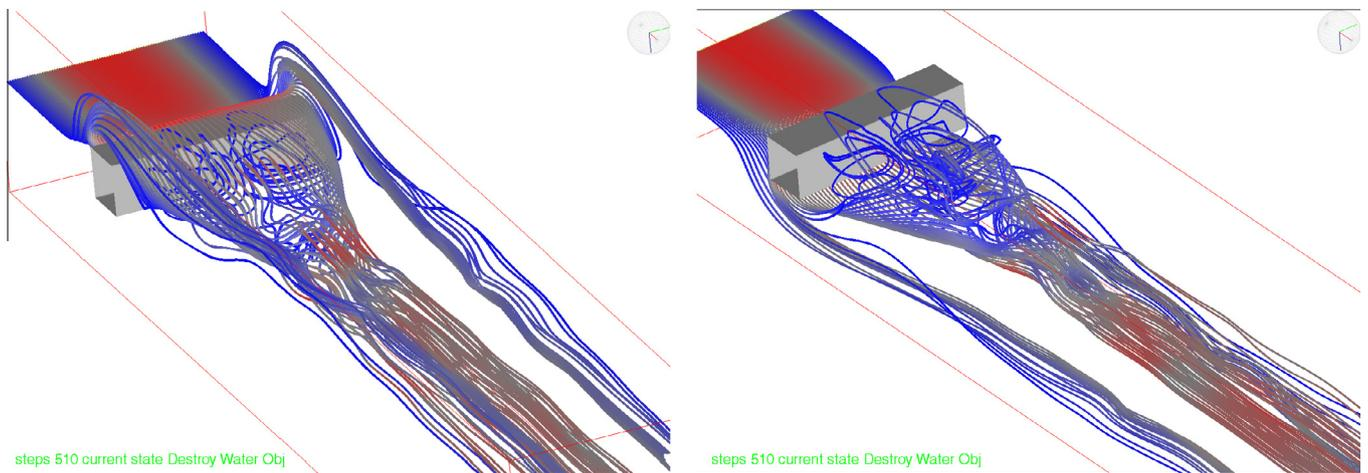
**Fig. 14.** Problem Q2: Streamlines of the developed flow around a square cylinder for  $Re = 100$ . The streamlines are selected for two fluid layers entering the domain slightly above and below  $x = 0.21$ .
