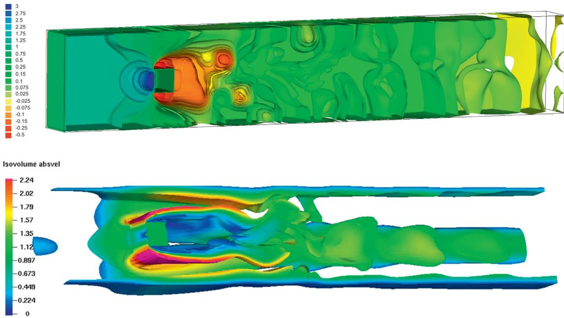
Fig. 15. Problem Q2 ( $Re = 100$ ): Pressure isosurfaces and vorticity isosurface  $|\mathbf{w}| = 20$  colored by the absolute velocity. The plots illustrate solution computed with  $h_{\max} = 1/256$  and  $h_{\min} = 1/1024$  at  $t = 16$ . (For interpretation of the references to color in this figure legend, the reader is referred to the web version of this article.)
