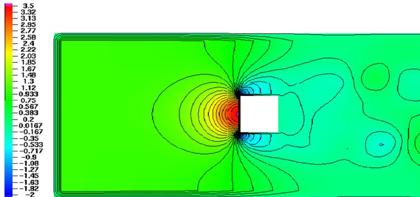
**Fig. 13.** Problem Q2 ( $Re = 100$ ): The midplane pressure contours around a square cylinder. The solution shown was computed with  $h_{\max} = 1/256$  and  $h_{\min} = 1/1024$  at  $t = 16$ .
