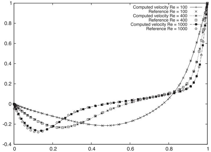
Fig. 6. Left: The 3D driven cavity problem setup; Right: The centerline  $((0.5, 0.5, z), 0 \leq z \leq 1)$   $u$ -velocities compared to reference data from [33].
