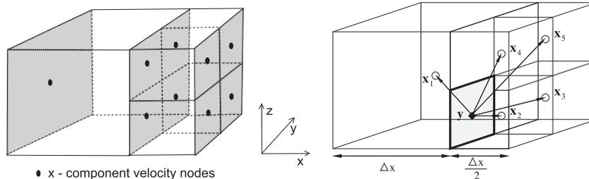
Fig. 1. Left: Each shared face holds a node for velocity  $x$ -component. The nodes are located at faces barycenters. Right: Discretization stencil for  $\partial p/\partial x$ .
