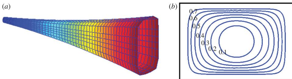
**Figure 4.** (a) The shape of the rods on the hairy sphere in figure 3*d*. (b) The cross section of the rod for a unit cell  $[0, 1.5] \times [0, 1]$  and various volume fractions. The number on each curve is the volume fraction of the inclusion. (Online version in colour.)
