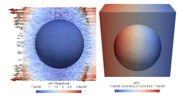
Velocity vectors colored with the velocity magnitude on the xz-section of  $\Omega^+$  and in  $\Omega^-$  (left) and pressure in  $\Omega^-$  and half  $\Omega^+$  (right).
