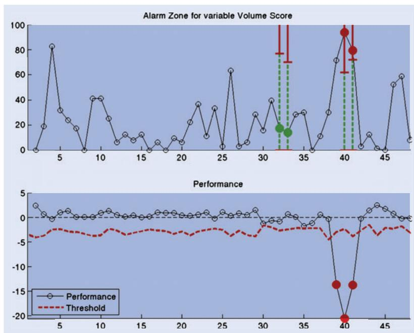
Figure 9. Auto adaptive alarm zones on the *Volume Score* explanatory variable for the order  $T(139)$  displayed in figure 3; Top: four alarm zones are active, two realizations of the *Volume Score* exceed the auto adaptive thresholds and thus emerge as a highly likely explanation for the bad performance exhibited by this order (see Bottom graph).
