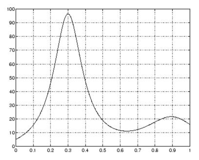
The graph shows that the function has a local minimum near x = 0.6. The function fminsearch finds the *minimizer*, the value of x where the function takes on this minimum. The first argument to fminsearch is a function handle to the function being minimized and the second argument is a rough guess at the location of the minimum:
