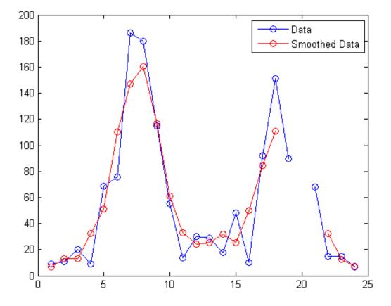
The extent of the smoothing is controlled with the variable span. The averaging calculation returns NaN values whenever the smoothing window includes the NaN value in the data, thus increasing the size of the gap in the smoothed data.
