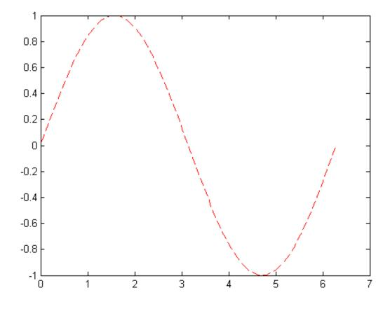
The 'r--' string is a *line specification*. Each specification can include characters for the line color, style, and marker. A marker is a symbol that appears at each plotted data point, such as a +, o, or \*. For example, 'g:\*' requests a dotted green line with \* markers.
