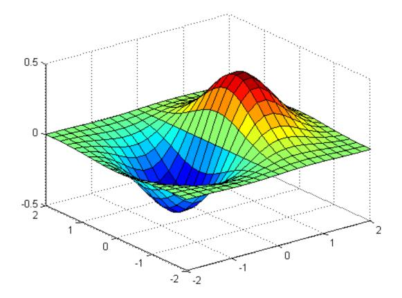
Both the surf function and its companion mesh display surfaces in three dimensions. surf displays both the connecting lines and the faces of the surface in color. mesh produces wireframe surfaces that color only the lines connecting the defining points.
