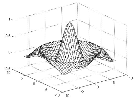
By default, MATLAB uses the current colormap to color the mesh. However, this example uses a single-colored mesh by specifying the EdgeColor surface property.
