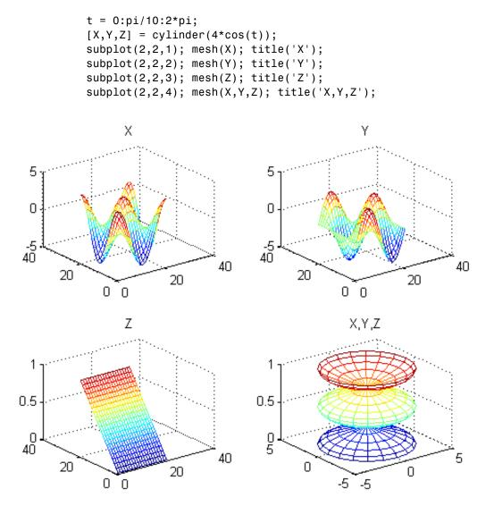
The first two inputs to the subplot function indicate the number of plots in each row and column. The third input specifies which plot is active.
