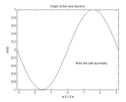
The location of the text string is defined in axes units (that is, the same units as the data). The annotation function enables you to place text in normalized figure units.
