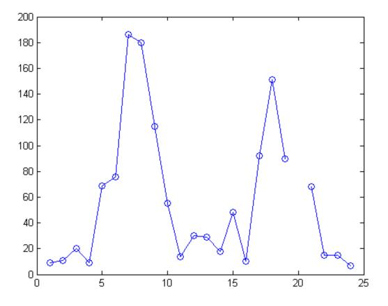
The NaN value at hour 20 appears as a gap in the plot. This handling of NaN values is typical of MATLAB plotting functions.
